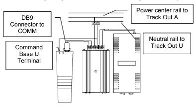
This diagram explains the connections to the back of the TPC3000 Series.
