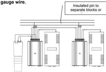
Wiring more than one TPC3000 Series to a layout is easy. It requires you to insulate the center rail of each loop or block of track. If the track is a continuous loop and you want to make two separate blocks, both ends must be insulated making the loop two separate sections. The above diagram shows the insulating pin location and the connections to the two TPC3000 Series.
