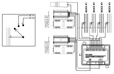
The second configuration for the BPC3000 has five positions: OFF, TPC1, TPC2, TPC3 and TPC4. It can route power from 4 different transformers to one block of track. In this configuration 2 of these rotary switches are in a BPC3000. This is called Four TPCs to two Blocks of track.
