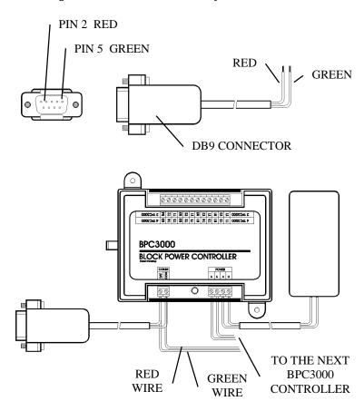
• Start by connecting the DB9 end of the cable to the
