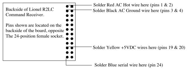
NOTE: When soldering the wires to these pins, please ensure the wires touch only the pins you are soldering them to, otherwise a short circuit will occur and could possibly cause permanent damage to your R2LC receiver.
