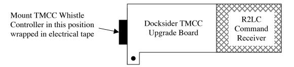
We strongly recommend wrapping the TMCC whistle Controller with electrical tape prior to mounting to the locomotive frame. This way you can protect the board from shorting out inside the locomotive. Use the double-sided tape to mount the board, providing you have adequate room.
