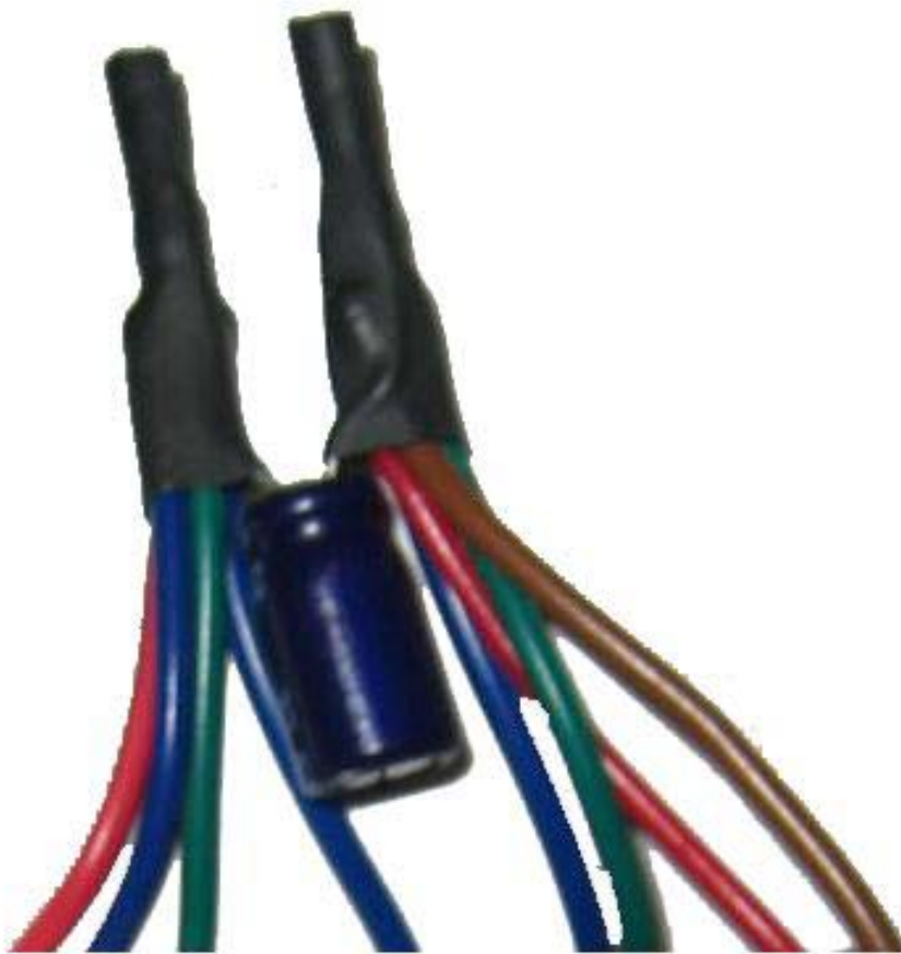
22uf / 25v capacitor installed on the motor wires
