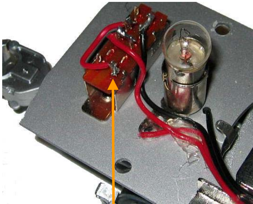
Solder lighting wire here from the shell
