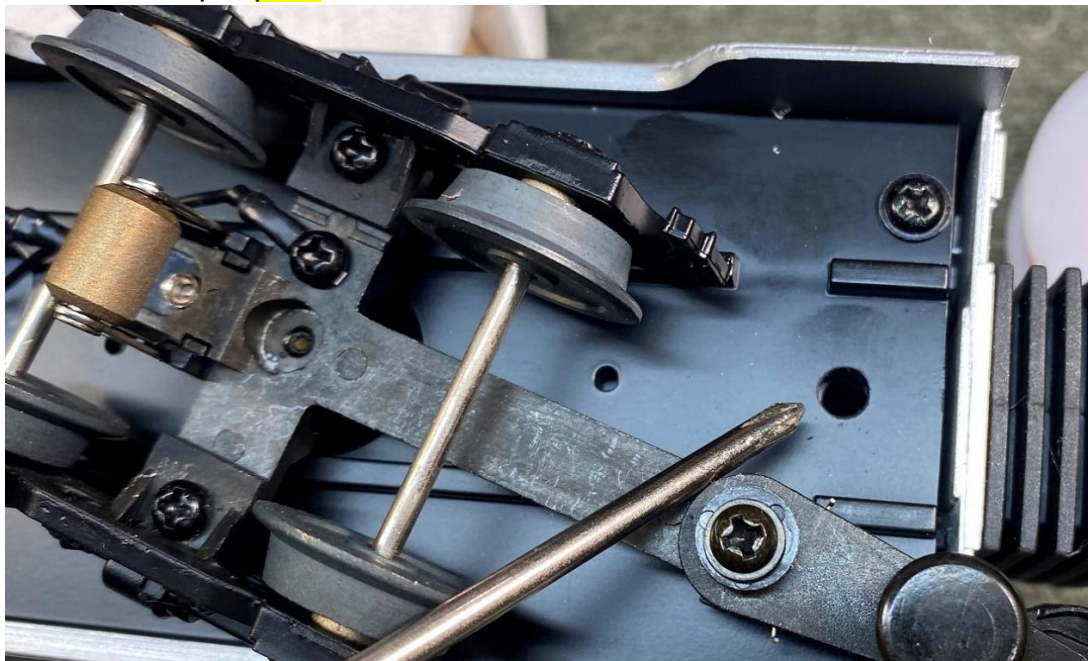
Pic 5: Optional pot adjustment access hole in floor; for Premier cars.
