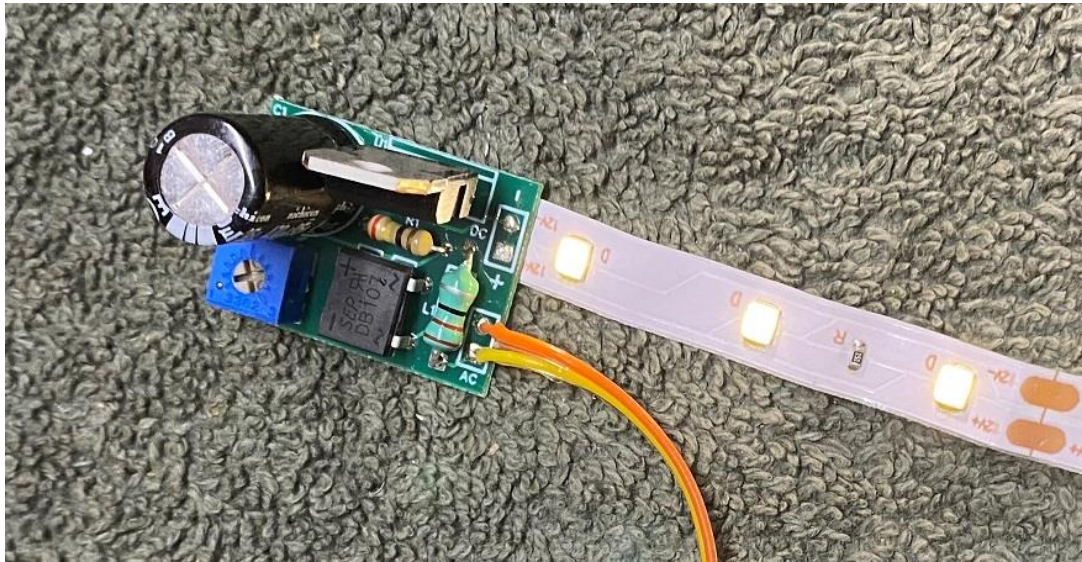
Pic1: Module soldered directly to led strip, being tested; for Premier cars.
