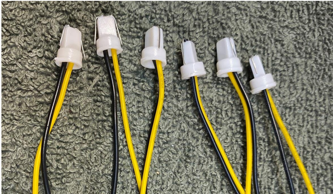
Pic 8: Typical batch of direct power connection pigtails using OEM bulb holders.
